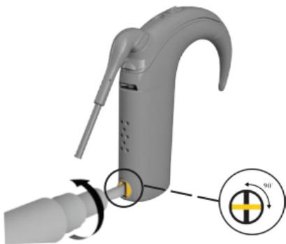
1. Turn the lock screw anticlockwise to unlock the tamper-resistant battery cover (clockwise to lock).
