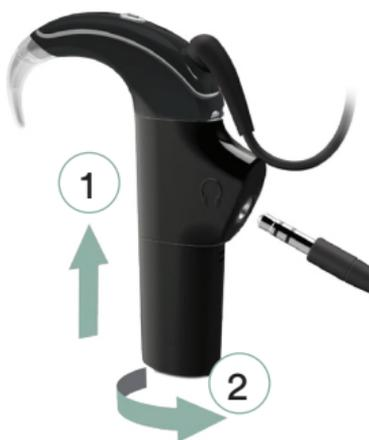
3. Insert the battery module, then twist to connect.
