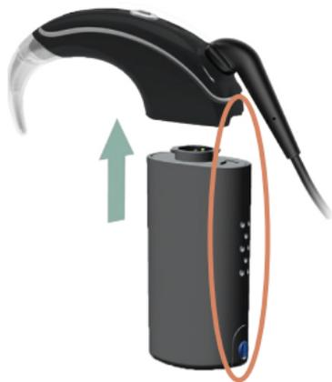
2. Twist the battery module as shown to attach the parts.
