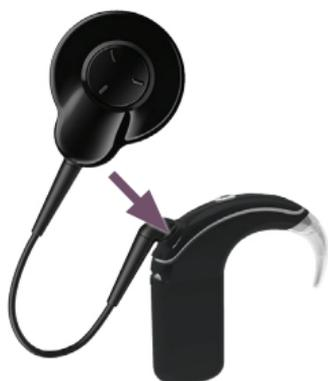
2. Push the new coil cable into the processing unit until it clicks into place.
