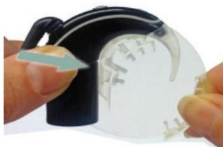
2. Attach the coil to the Headworn Adaptor.
