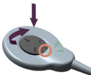
3. Insert the new magnet and turn clockwise until it stops.
