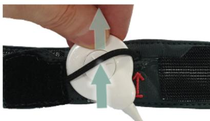
4. **Pull** the coil cable sideways through the elastic loop.
