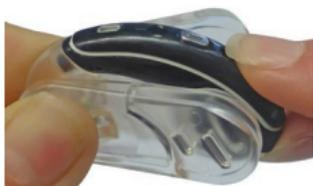
Orient the sound processor so it faces the same way as when it is worn on the ear.
