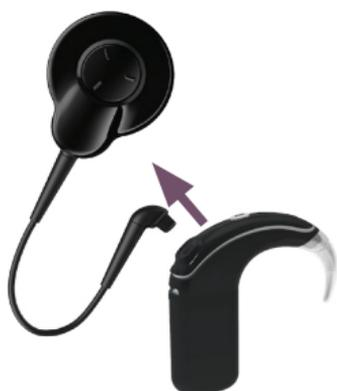
1. Hold the coil cable grip and firmly pull it straight out of the processing unit. Do not pull on the flexible part of the coil cable.
