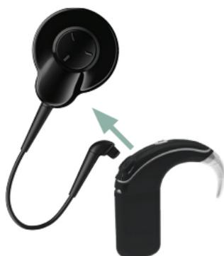
1. Hold the coil cable grip and firmly pull it straight out of the processing unit. Do not tug on the flexible part of the coil cable.
