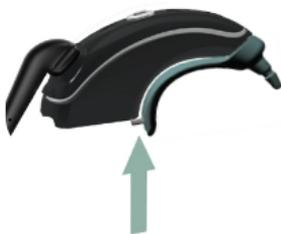
3. Attach the battery module and attach the earmould.
