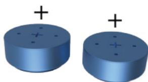
5. Insert the batteries into the battery holder with the flat side (positive terminal) facing up.
