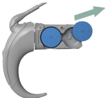
3. Remove the batteries from the battery holder.
