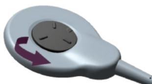
1. With finger grips facing up, unscrew the magnet anticlockwise.
