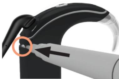
1. Push the lock to the far left to lock the battery module.
