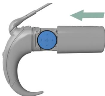
6. Replace the battery cover by sliding it up towards the processing unit.
