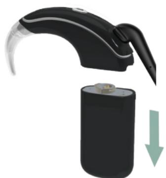
2. Pull the battery module from the processing unit.
