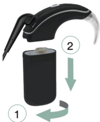
1. Twist to disconnect, then remove the battery module.
