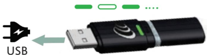
4. The LED changes to steady green when the module is fully charged.
