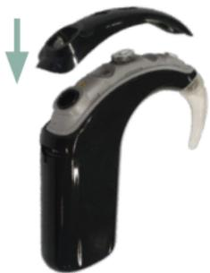
1. Fit the replacement microphone cover onto the processing unit.
