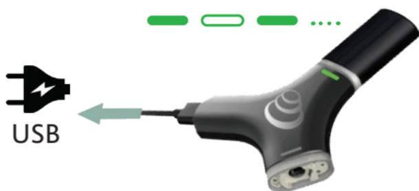
3. The LED changes to steady green when the module is fully charged.
