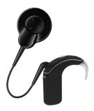
If you use a disposable battery module instead of a rechargeable battery module, or use the processing unit with an acoustic component worn in the ear, it is protected against failure from dust and splashing water (IP54 rated).
