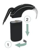
Twist to disconnect, then remove the battery module.
