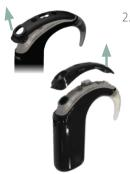
2. Lift the microphone cover from the bottom edge, then lift it to remove.
