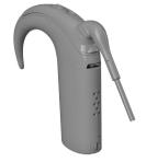
Press and hold the button for 5 seconds, then release to turn off your sound processor.
