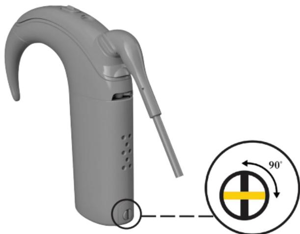
**LOCK** Turn the locking screw **clockwise** with the battery cover locking tool until it is in a **horizontal** position.
