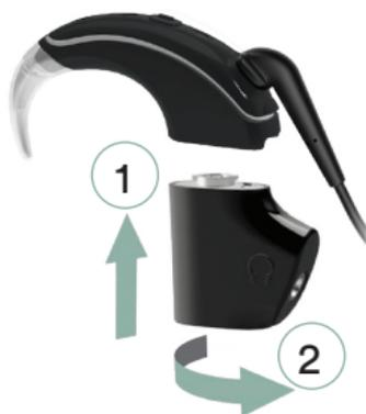
2. Insert the monitor earphone adaptor, then twist to connect.
