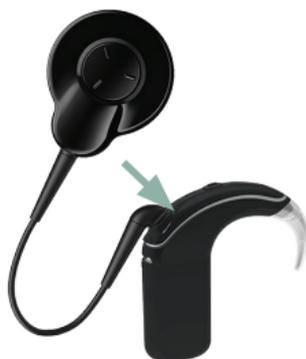
3. Push your coil cable into the processing unit until it clicks. **Do not twist.**
