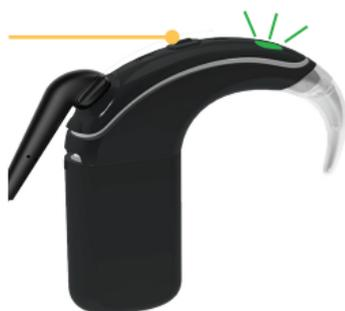
Each button press cycles you through telecoil (if enabled), and then your wireless accessories (in the order in which they were paired to your sound processor).
