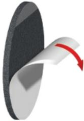
1. Peel off the single backing strip on the adhesive side of the pad.
