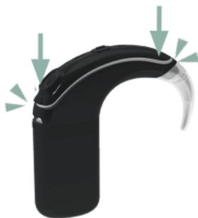
2. Press down firmly with a finger on each end of the microphone cover until you feel a click.
