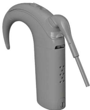
1. **Press and hold** the button for 5 seconds, then **release** to turn off your sound processor.
