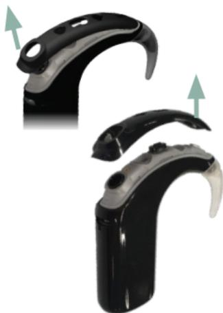
2. Lift the microphone cover from the bottom edge, then lift it to remove.
