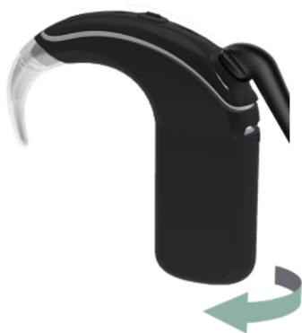
1. Twist the battery module as shown to release it from the processing unit.
