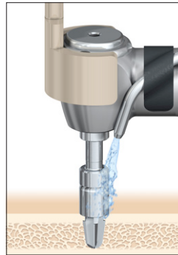
Fig.14: Drilling with Guide drill with spacer removed
