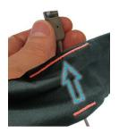
4. If the socket cover is in place on the back of your processor, remove the socket cover.
