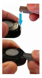
Insert your processor into the pocket, making sure that the back of the processor (with magnet) is facing towards you.
