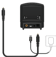
Typical connection to TV (Toslink cable)
