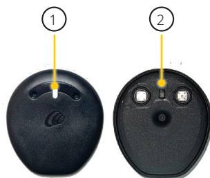
1. Microphone cover LED lens 2. Sound processor LED light indicator
