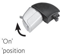
Figure 24: Oticon receiver connected to the Euro Accessory Adaptor
