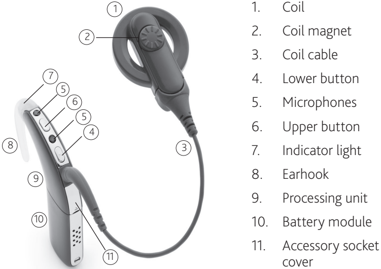
Figure 1: CP810 Sound Processor parts
