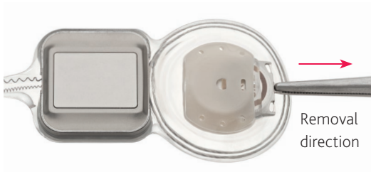
Figure 34: CI632 implant, cassette removal using metal tab
