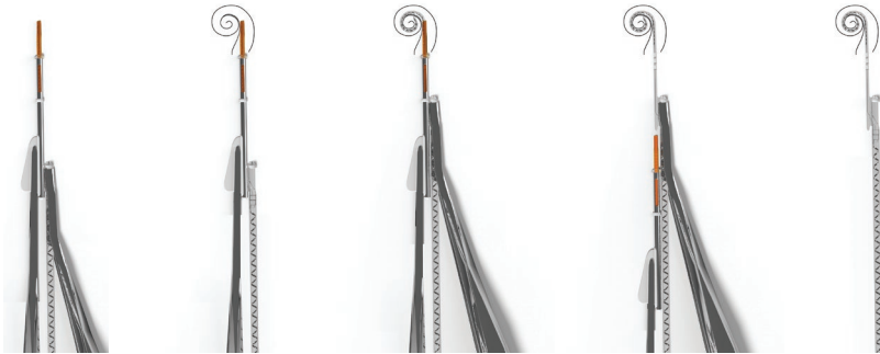
Figure 10: Steps for inserting electrode into the cochlea
