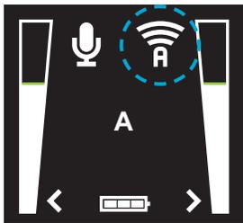
Connected to streaming device.
