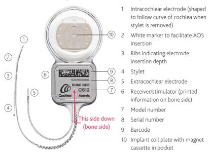
Figure 2: CI612 cochlear implant with Contour Advance electrode (bone side)
