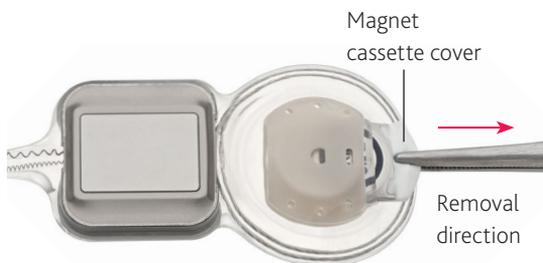
Figure 20: CI600 Series implant with magnet cassette partially removed
