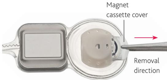
Figure 15: CI600 Series implant with magnet cassette partially removed
