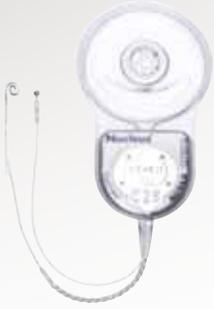
The Freedom implant, commercially launched in 2005, has improved electronic capabilities compared with previous implants. Significant advantages include the availability of telemetry enabling new AutoNRT™ functionality. The Freedom implant has the same small physical packaging and accrues the same surgical benefits as the CI24R implant. In addition, the Freedom implant was strengthened to protect the sensitive electronics against external impact.
