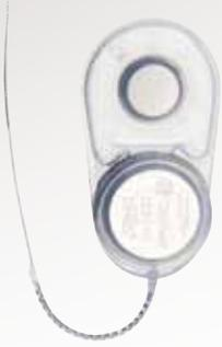
The CI22M implant, released in 1985, was Cochlear's first commercial implant. In 1986, the CI22M was released with an internal magnet to hold the external transmitting coil in place.
