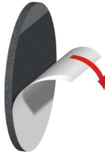
2. Attach the pad to the back of the processor—press down firmly.
