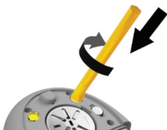
5. **Firmly push**, and then turn the tool 90° clockwise.
