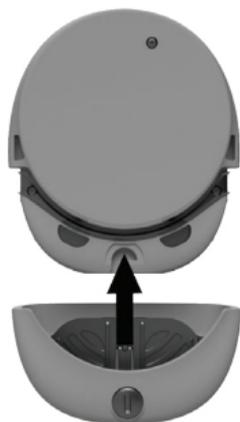
6. Replace the battery cover. Lock the cover if required. Your processor will automatically turn on.
