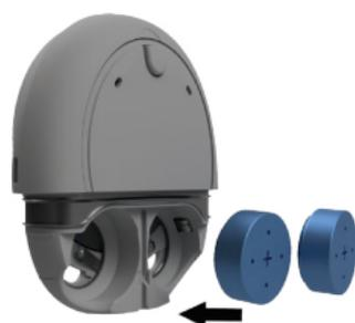
5. Insert the batteries into the battery holder with the side with holes on it (positive terminal) facing out.
