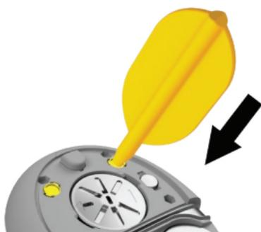
4. **Firmly push** the tip of the removal tool into the middle of the microphone protector.
