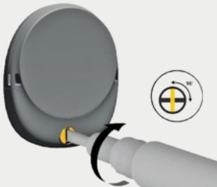
1. To lock, turn the locking screw clockwise with the battery cover locking tool until it is horizontal.
