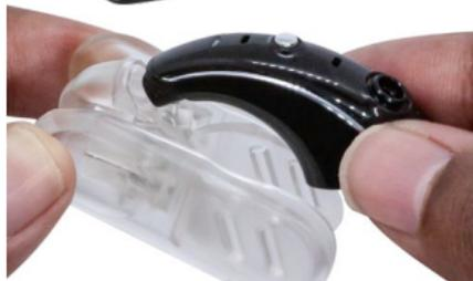
3. Push down on the top of the processing unit when attaching the battery module, to ensure the metal tab on the Koala Clip fits inside the processing unit case.
