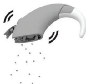
Your processing unit is protected against failure from dust and immersion in water at depths of up to 1 metre (IP68 rated) when you wear it with:
