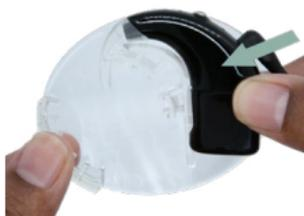
2. Attach the coil to the Headworn Adaptor.
