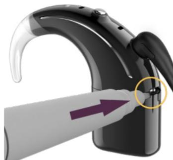
2. Push the lock to the far right to unlock the battery module.
