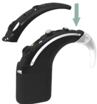
2. Press down firmly with a finger on each end and the middle of the microphone cover until you feel a click.
