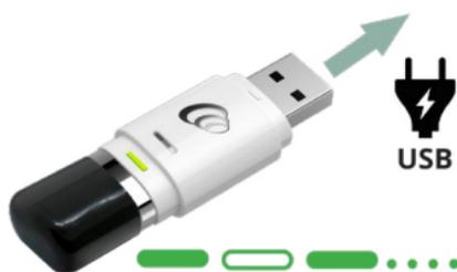
4. The LED changes to steady green when the module is fully charged.
