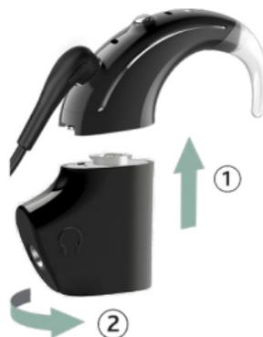
3. Insert the battery module, then twist to connect.
