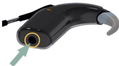
Slide the cover off the sound processor.
