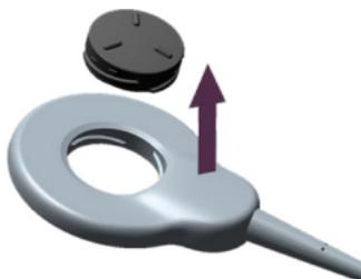
3. Insert the new magnet and turn clockwise until it stops.
