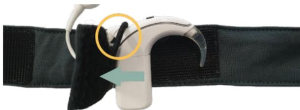
6. Close the flap over the processor (press firmly).
