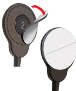
3. Peel off the two semicircle backing covers on the cushion side of the pad.
