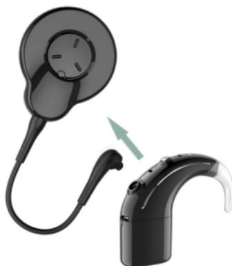
2. Push the new coil cable into the processing unit until it clicks into place. **Do not twist.**
