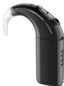
1. Press and hold the button for 5 seconds, then release to turn off your sound processor
