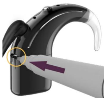
1. Push the lock to the far left to lock the battery module.
