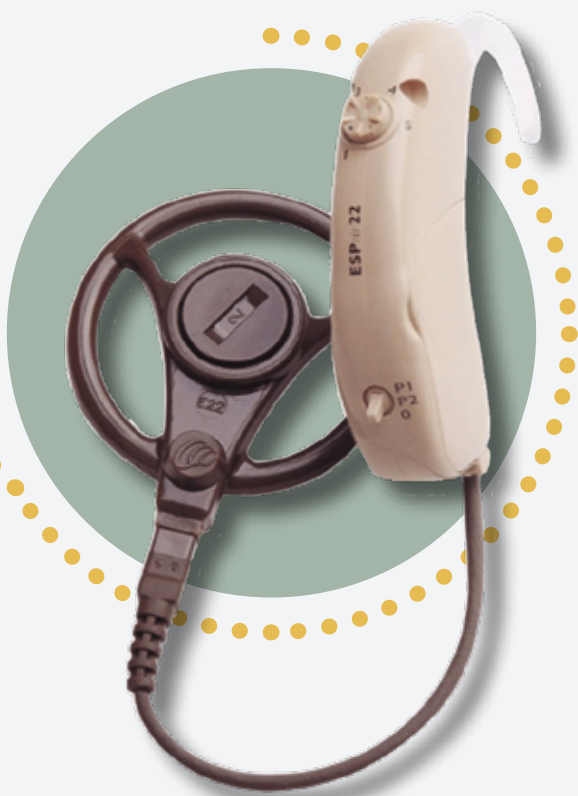
The Cochlear Esprit Sound Processor for Nucleus 22 recipients, released in 2004
