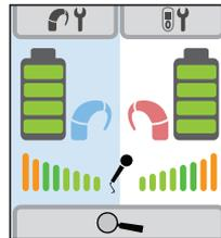
Figure 34: Bilateral mode processor battery status screen
