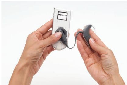
Figure 12: Placing the coil on the coil sensor guides
