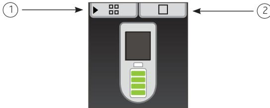
Figure 16: Accessing Advanced mode (1) or Simple mode (2)
