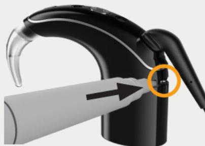
2. Push the lock to the far right to unlock the battery module.
