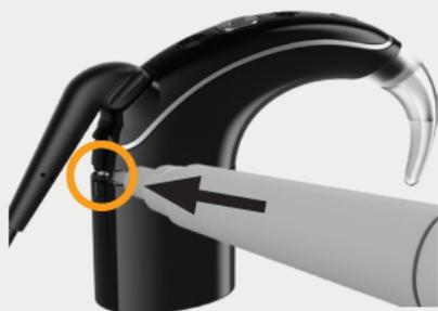
1. Push the lock to the far left to lock the battery module.
