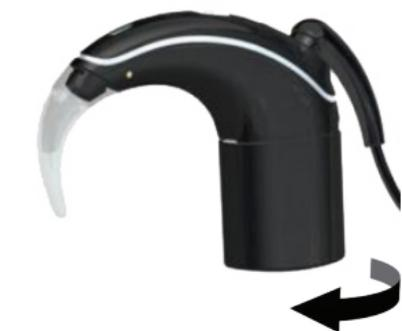
1. Twist the battery module as shown to release it from the processing unit.
