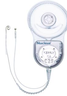
The CI24R Implant was released in 2000 with perimodiolar (Contour Advance®) and straight electrodes. Within 21 years, the CI24R Implant has a combined Cumulative Survival Percentage of 97.23%.
