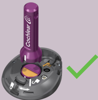
Correct position of the magnet in the sound processor
