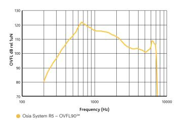
Measured on skull simulator TU1000 and compensated for skull impedance. Also compensated for actuator position based on: Transmission properties of bone conducted sound: measurements in cadaver heads, Stenfelt S, Goode RL, The Journal of the Acoustical Society of America 2005 Oct;118(4):2373-91.
