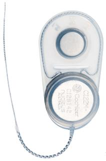
The CI22M implant, released in 1985, was Cochlear's first commercial implant. In 1986, the CI22M was released with an internal magnet to hold the external transmitting coil in place.
