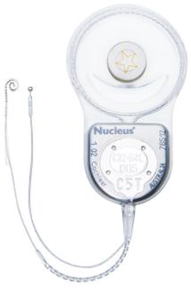
Commercially released in 2005, the CI24RE introduced a new integrated circuit with a mechanical design and production processes based on the proven architecture of the CI24R implant. The new integrated circuit substantially increased the capability and future-readiness of the system. Features include AutoNRT™, numerous stimulation modes and native compatibility with the Nucleus CP810 Sound Processor and CR110 Remote Assistant.
