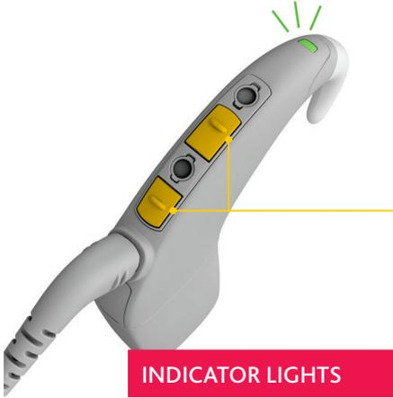
Short-press and release both buttons at the same time to lock and unlock the processor.
