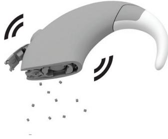
If sand or dirt ever enter the processor, shake the components carefully to remove it and change the microphone protectors.
