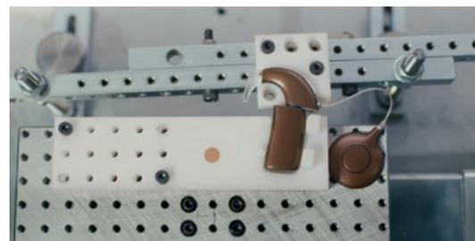
Sound processor battery compartment test – 6,000 cycles
