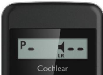
If your processor is out of range or experiencing interference, the remote control displays dashes (shown at left).
