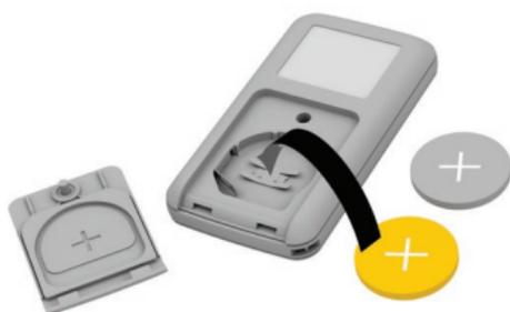
3. Insert the new battery. Make sure the plus sign “+” is facing up. Take care not to damage the battery contacts.
