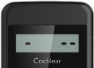
If your remote control is not paired to any processor, it displays dashes (shown left) and "blinks" when you press buttons.
