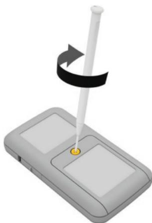
5. Lock the battery cover in place by turning the screw clockwise with a small Phillips head screwdriver until tight.
