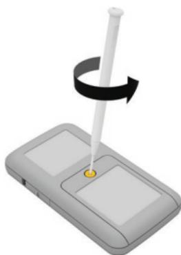
1. Unlock the battery cover by turning the screw anticlockwise with a small Phillips head (cross-head) screwdriver.
