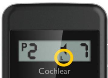
4. The remote control then shows successful pairing of either left (L) or right (R) processor.
