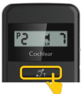
2. To stop streaming audio, short-press the telecoil button. The accessory icon will disappear.
