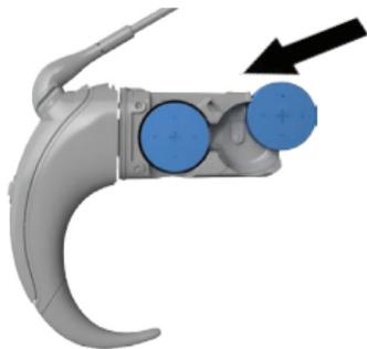
3. Insert two new 675 (PR44) zinc air disposable batteries (not silver oxide or alkaline), flat side facing up.
