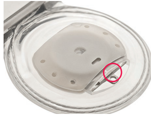
Figure 22: CI600 Series implant - metal tab on magnet cassette
