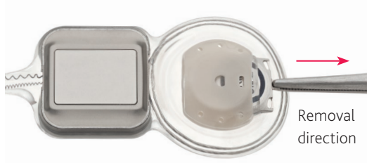
Figure 18: CI600 Series implant - magnet cassette removal using metal tab
