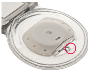
Figure 17: CI600 Series implant - metal tab on magnet cassette
