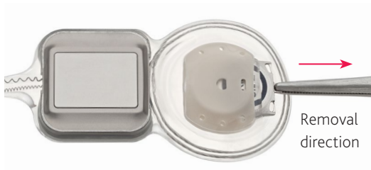
Figure 23: CI600 Series implant - magnet cassette removal using metal tab
