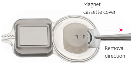
Figure 21: CI600 Series implant with magnet cassette partially removed
